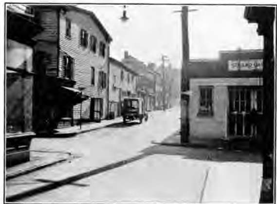
The offset intersection at Spring Alley and Church Street reduces the traffic capacity of the intersection; it also causes frequent collisions.
